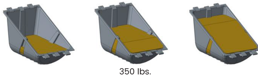
Figure 7. - Ballast Weight Chart
